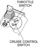
Figure 13. Throttle Switch
